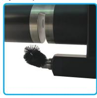
The Hydro-Wiper is an external anti-fouling system fully integrated with the SUNA V2 nitrate sensor. The Hydro-Wiper keeps the SUNA V2 sample windows clean for several months and is specifically intended for use in freshwater and coastal systems.
