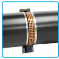
The SUNA V2 anti-fouling guard is a semi-circular piece of perforated copper attached to a plastic armature that fits into the sample chamber. It provides passive fouling prevention through the release of copper ions that inhibit biological growth in the area. The anti-fouling guard is a reliable and affordable approach to increase deployment time and decrease operating costs. It is intended for use in blue-ocean applications with low-to-no suspended sedimentation and/or low-to-no turbidity.
