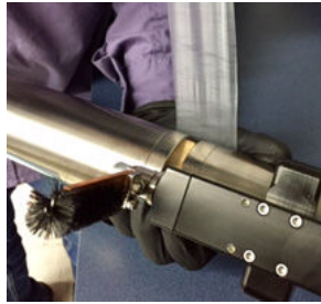
Figure 1 Parafilm® to be wound around optical area
