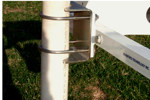
Figure 2.1 Installing Mounting Bracket & U-Bolts
